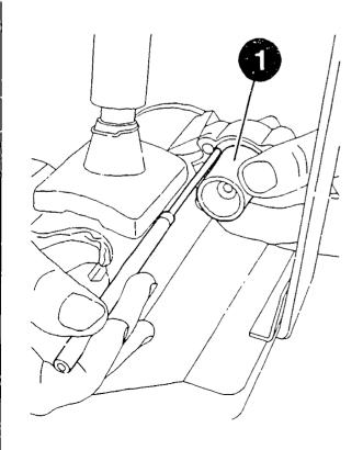
Disassembling bearing-end plate
